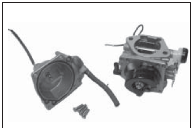
Figure 5-17. Fuel Bowl Removed from Carburetor.
